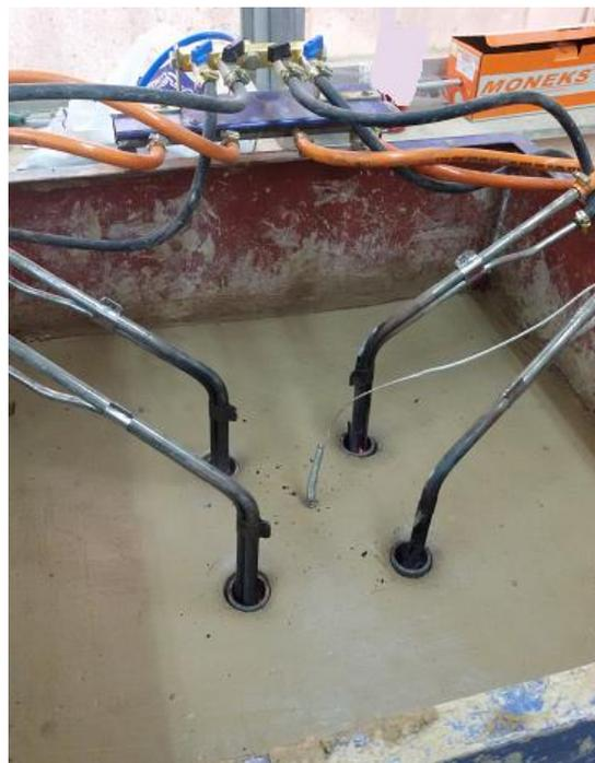
**Plate 2. Heating system inside casing to during soil improvement.**
