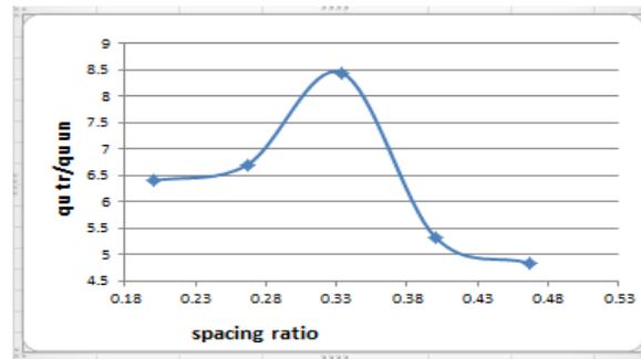
**Fig. 6. Variation of bearing improvement ratio versus Spacing ratio.**
