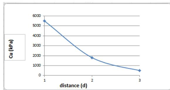
Fig. 5. Relationship between undrained shear strength and distance.
