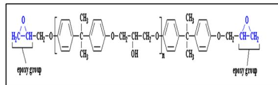
**Fig.1. The structure of epoxy groups [10].**
